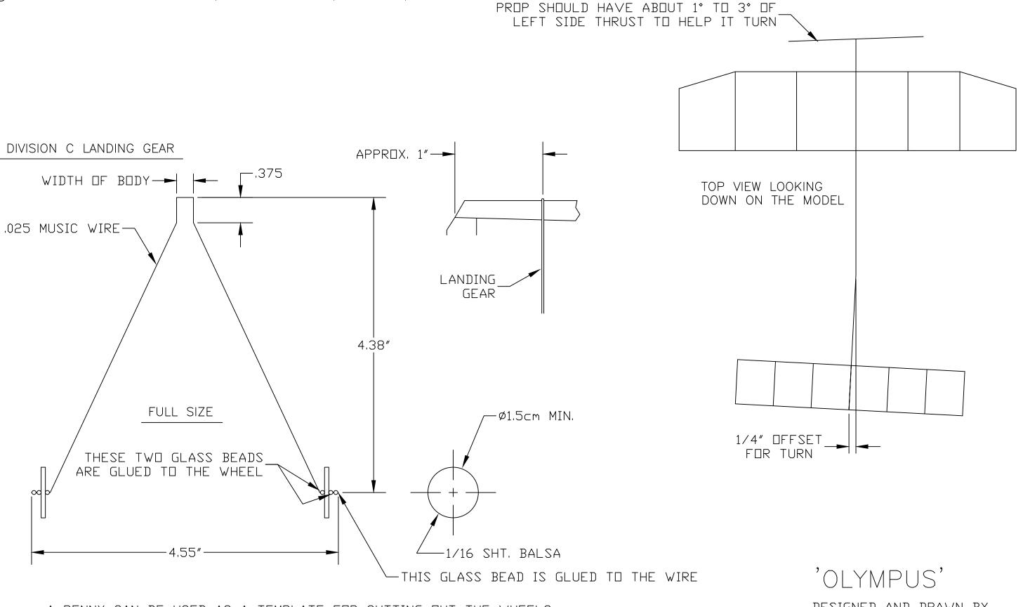
A PENNY CAN BE USED AS A TEMPLATE FOR CUTTING OUT THE WHEELS
